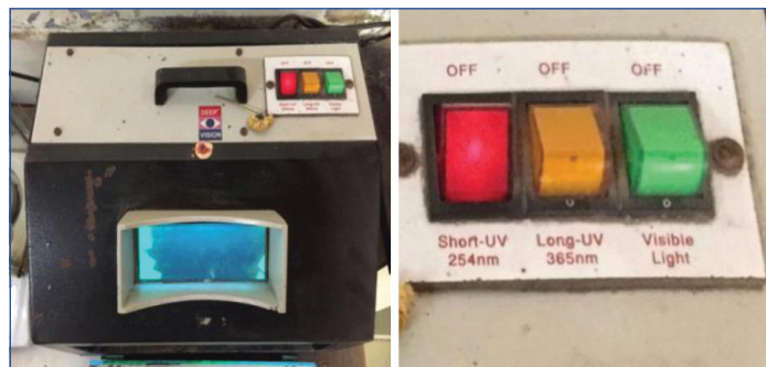
[Table/Fig-2]: UV chamber used for Photofunctionalization.
